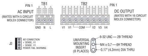
INPUT & OUTPUT CONNECTIONS: 6-32 SCREW WIRE CLAMPS ON 0.312" (7.9mm) CENTERS,
